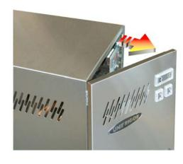
The new cover motor sheet with side opening similar to one door but with light narrow hinges and magnet locking, make easier to access the motor unit area and especially to the condenser, to facilitate regular cleaning operations. Moreover the thermostat and the pushbuttons, are fixed in the upper part of the motor unit area, a safe area without humidity, in order to preserve their functionally and their duration in time.
